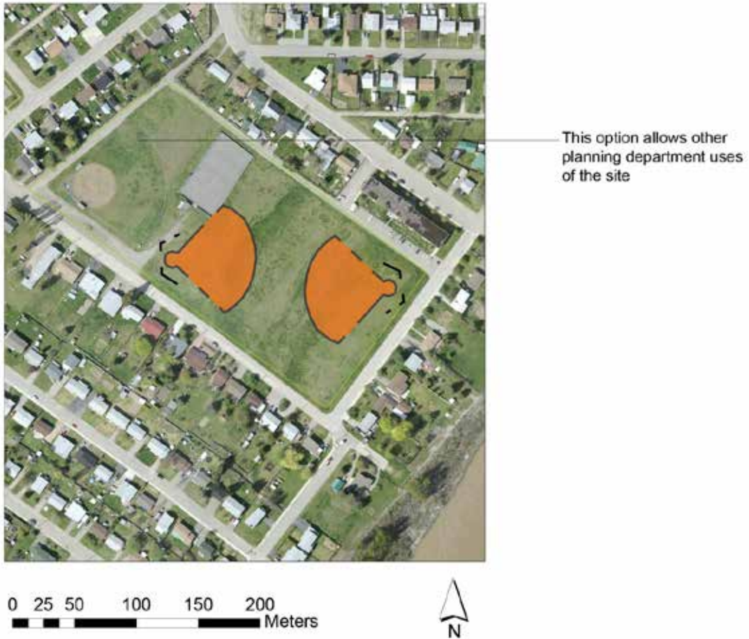
Figure 11: Option 2 - Cariboo Field: Two softball diamonds - decommission existing ball diamond, relocate ball diamonds to floodplain
